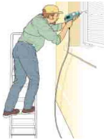
Figure 2a Incorrect - steps side-on to work activity
