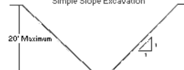
TYPE B SOIL Simple Slope Excavation
